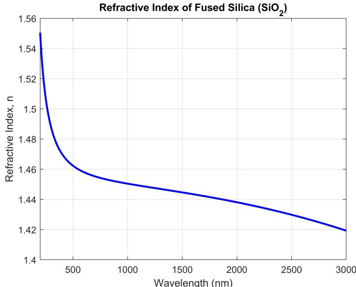
(b) Plot the group index  $n_g$  and the group velocity dispersion  $\beta_2$ . It is preferable to base the derivation on an equally spaced **frequency** grid. Remember: that the group index is most conveniently written in terms of frequency and is given by  $n_g = \frac{d\beta}{d\omega} c$ , with  $c$  the speed of light. And that the GVD is given by  $\beta_2 = \frac{d^2\beta}{d\omega^2}$
