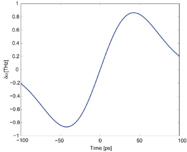
It can be shown from figure (also by derivation of  $\delta\omega(t)$ ), that the maximum frequency chirp is experienced at  $t = \pm 42.4 \text{ ps}$  leading to  $\delta\omega_{max} = \pm 0.86 \text{ THz.}$
